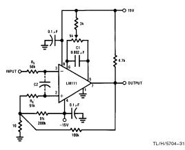
FIGURE 3. Positive Feedback with High Source Resistance
