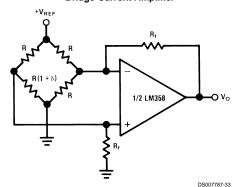
For  $\delta$  << 1 and  $R_f>>\,R$  $V_{O} \cong V_{REF} \left(\frac{\delta}{2}\right) \frac{R_{f}}{R}$
