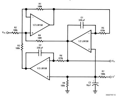
$f_0 = 1 \text{ kHz}$  Q = 50 $A_V = 100 \text{ (40 dB)}$
