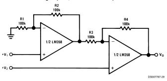
For  $\frac{R1}{R2} = \frac{R4}{R3}$  (CMRR depends on this resistor ratio match)  $V_O = 1 + \frac{R4}{R3} (V_2 - V_1)$  As Shown:  $V_O = 2 (V_2 - V_1)$
